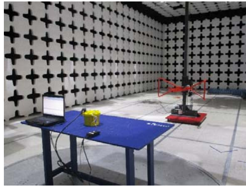
Radiated Emission Test setup (<1GHz) – Rear View
