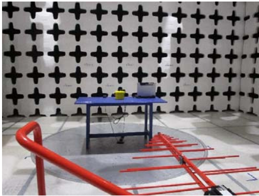
Radiated Emission Test setup (<1GHz) – Front View
