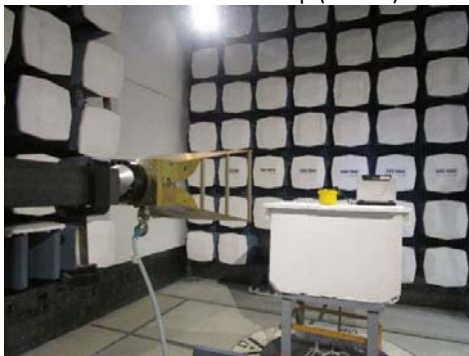
Radiated Emission Test setup (>1GHz) – Front View
