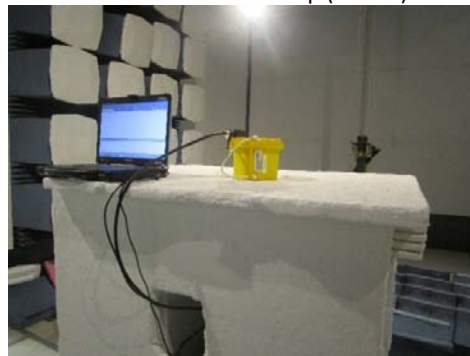
Radiated Emission Test setup (>1GHz) – Rear View
