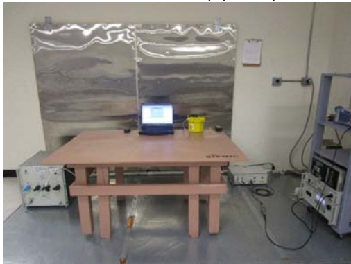
AC Line Conducted Emissions – Front View
