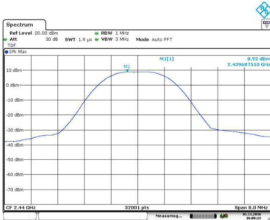
Figure 1: Conducted power (ch mid)
