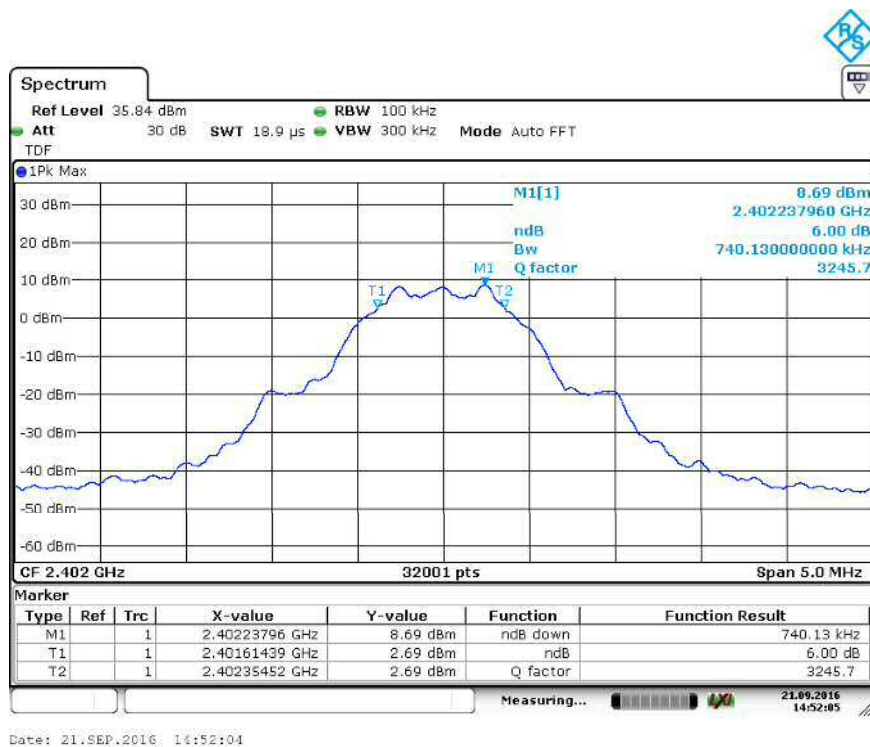
Figure 8: 6 dB bandwidth channel low
