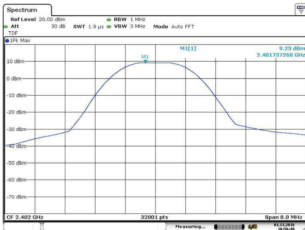
Figure 1: Conducted power (ch low)
