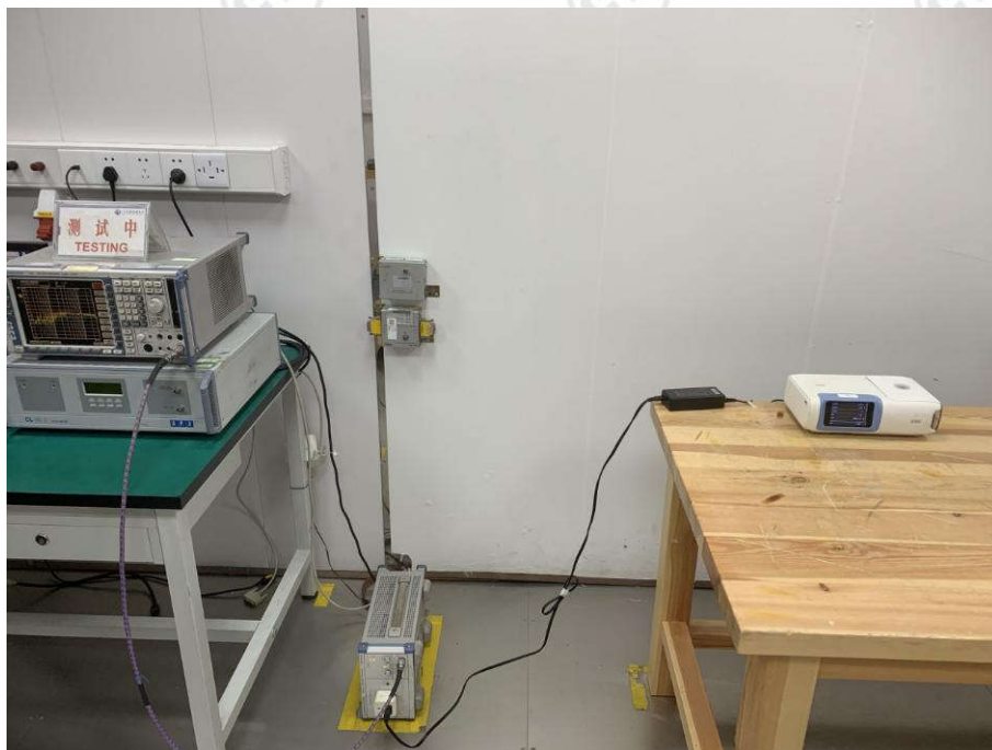
Conducted Emissions Test Setup
