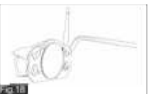
Figure14/Figure15/Figure16: Take out the base from bracket housing Figure17/Figure18: Insert magnet into base
