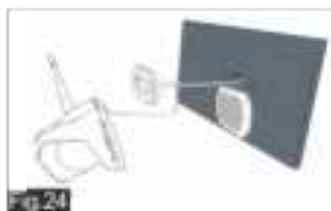
Figure24/Figure25: Put back the rear light and magnet the camera on metal plate.
