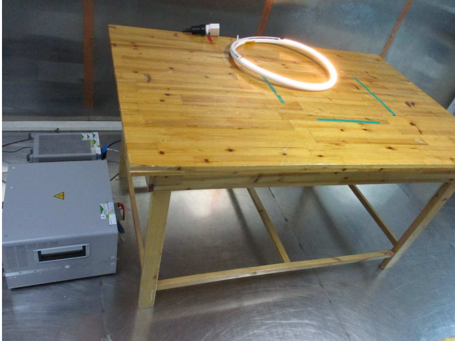
Photograph 1: Set-up for measurement of conducted emission
