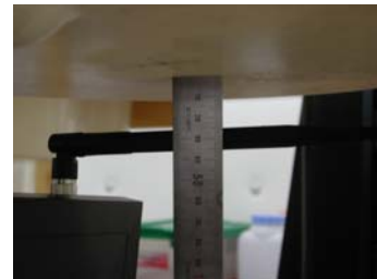
Fig. 21. Body SAR Test Setup with Holster
