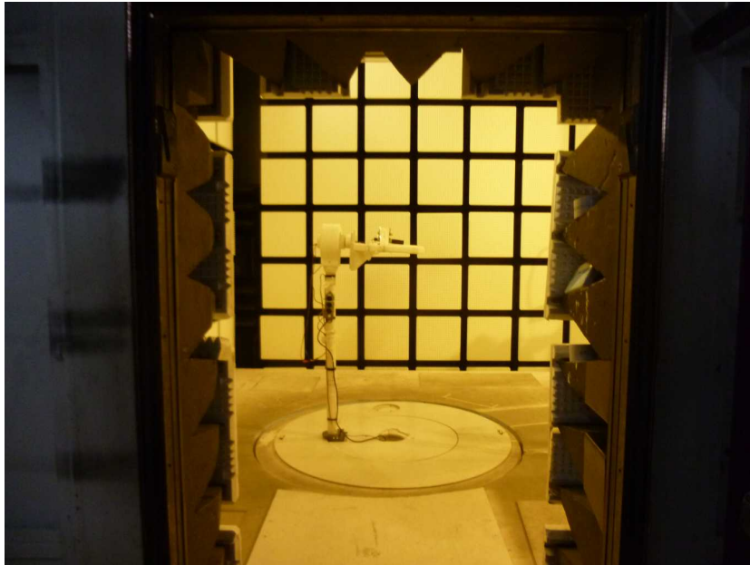
Photo 1: EUT with cast housing at the anechoic chamber
