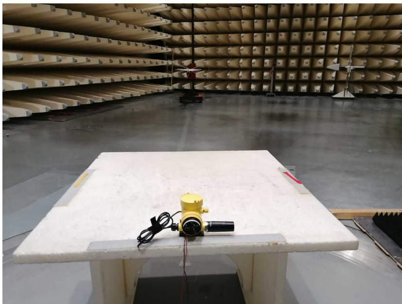
Photo 22: EUT with plastic housing at the semi-anechoic chamber
