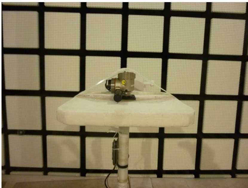
Photo 4: EUT with cast housing at the anechoic chamber
