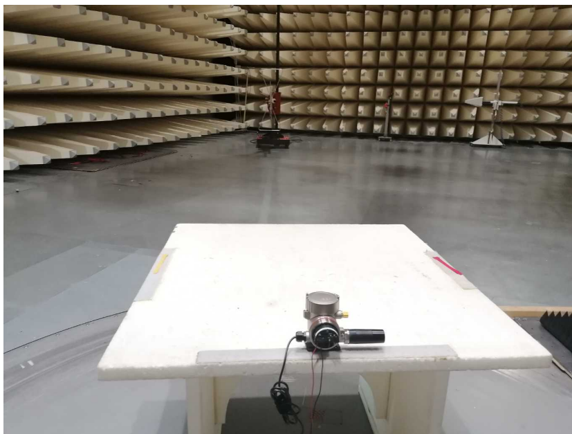
Photo 20: EUT with cast housing at the semi-anechoic chamber
