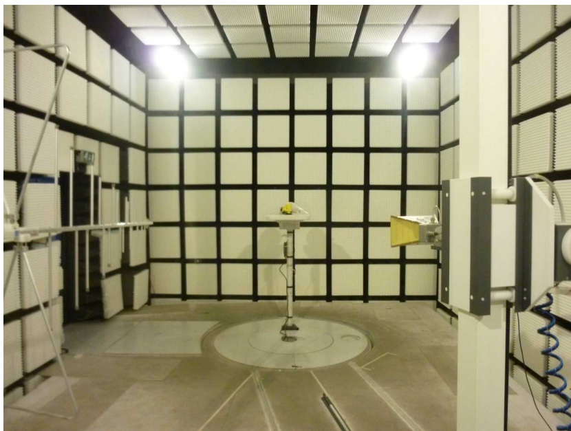
Photo 12: EUT with plastic housing at the anechoic chamber
