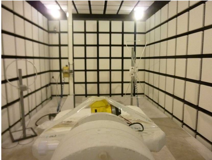
Photo 15: EUT with aluminium housing at the anechoic chamber
