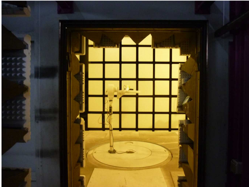
Photo 7: EUT with plastic housing at the anechoic chamber
