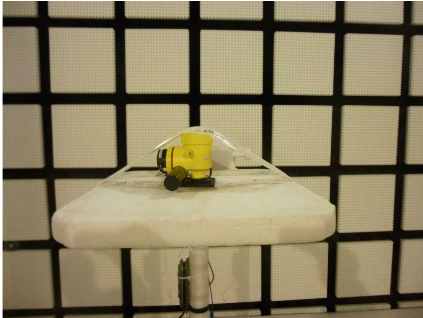
Photo 9: EUT with plastic housing at the anechoic chamber
