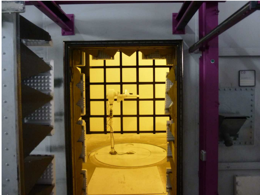
Photo 13: EUT with aluminium housing at the anechoic chamber
