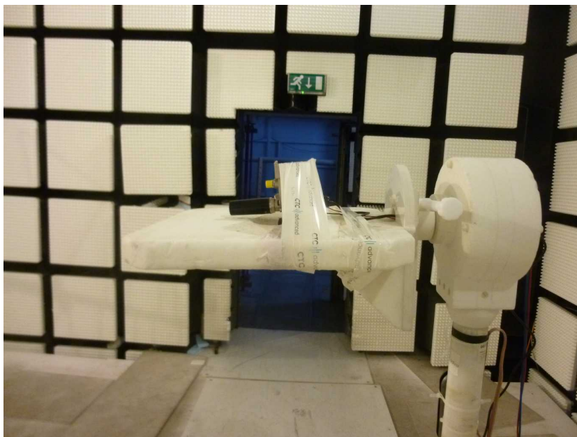
Photo 2: EUT with cast housing at the anechoic chamber
