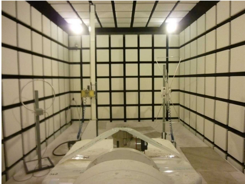
Photo 5: EUT with cast housing at the anechoic chamber
