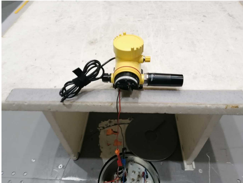
Photo 21: EUT with plastic housing at the semi-anechoic chamber
