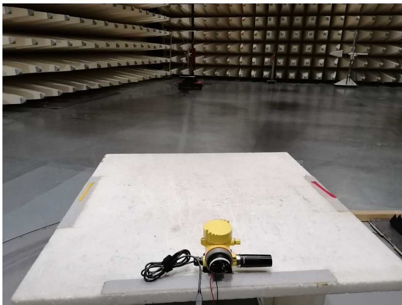
Photo 24: EUT with aluminium housing at the semi-anechoic chamber
