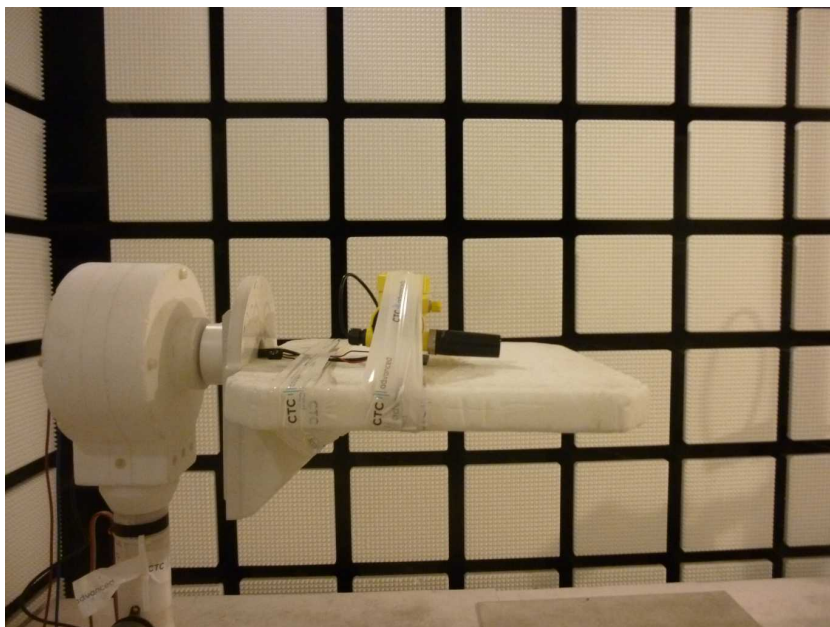
Photo 10: EUT with plastic housing at the anechoic chamber
