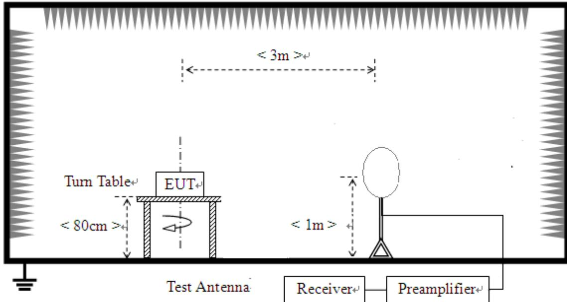
For radiated emissions from 30MHz to 1GHz
