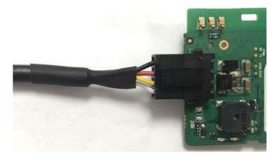
The picture above shows the 4 wire power and I/O harness. The wiring details are:
