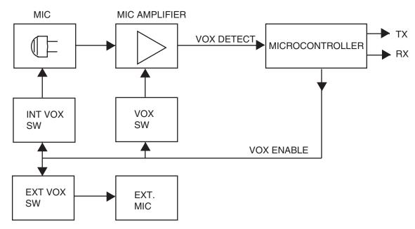
VOX control signal comes from MCU (U102) pin 75 (VOX enable). When VOX is activated, VOX enable (pin 75) is low, it will turn on VOX switch (Q102, Q103) to make microphone (MK101) and MIC amplifier (U104) in stand-by mode. When VOX signal is sent from MIC amplifier through R114 applied to MCU VOX detect (pin 38), for sampling reference level to change TV (TX control Voltage) or RV (RX control voltage) state.
