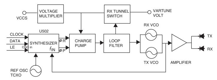
The frequency generation circuit is composed of synthesizer chip (U502) and voltage control oscillator (VCO) and voltage multiplier.
