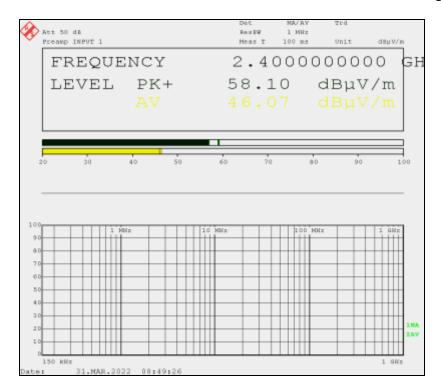
Legrand WNACB4 and Model WZ3ACB4 Zigbee Radio Zigbee Radio transmitting Ch 11 2405 MHz O-QPSK Vertical Polarity
