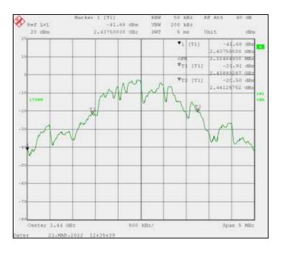
Legrand WNACB4 and WZ3ACB4 Zigbee Radio Mid channel 18, 2440 MHz, O-QPSK Modulation
