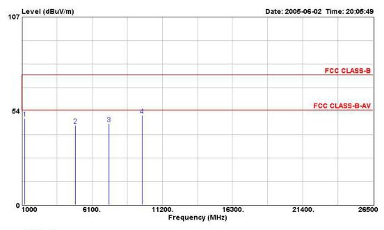
:03СНОЗ-НҮ Site Condition: FCC CLASS-B 3m HORN-ANT-6741-200505 HORIZONTAL EUT :SpeedTouch 585(i)v6 :120V/60Hz Power Mode 1 : ST585(i)v6 Memo :TX CHO6 2437MHz 11b Over Read Limit Cable Preamp Freq Level Limit Level Line Factor Loss Factor Remark MHz dBuV/m dB dBuV dBuV/m dB dB dB 1 1214.000 49.30 -24.70 63.31 74.00 -14.01 1.33 40.09 Peak
