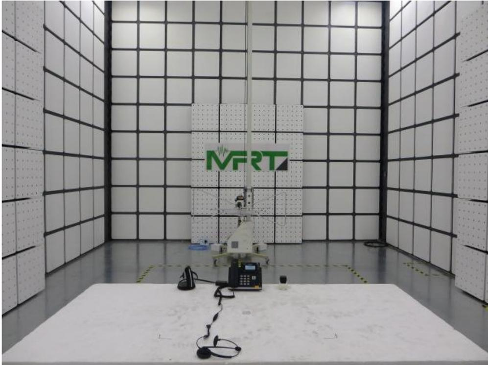
Test Mode 1: Power by adapter #1 and Communication with another IP Phone
