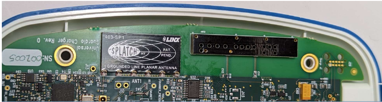
Internal Picture 3: Antennas present on the main board. 403MHz MICs antenna is Linx Technologies ANT-403-SP (left). LTE antenna is YC0003AA from Quectel Wireless (right). LTE module is utilized by LTE modem on the bottom of the PCB which is a certified module under FCC ID: 2AY43-EG25G.
