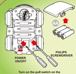
Turn on the pull switch on the car bottom to the ON position (open), and the OFF position is (closed);
