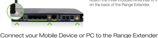
Attach the three included Antennas to the connectors
