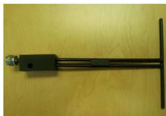
Figure 1 – MVG COMOSAR Validation Dipole
