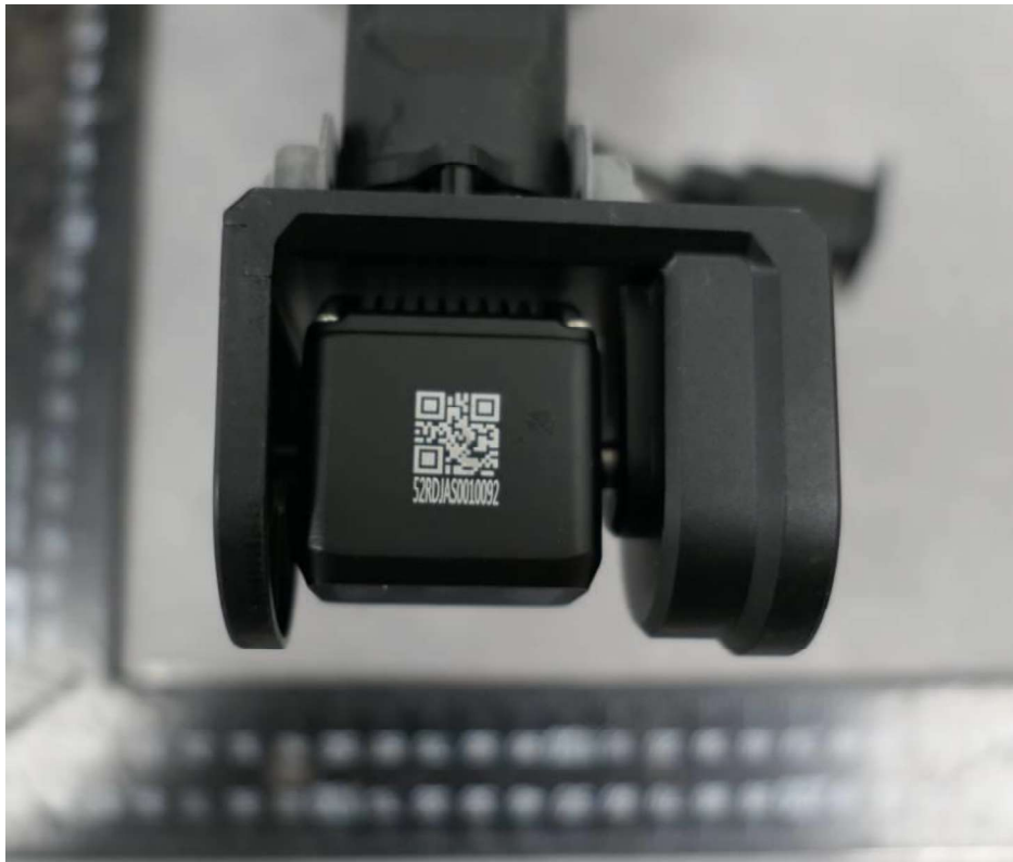
Fig. 28: FPV camera view (for both models)
