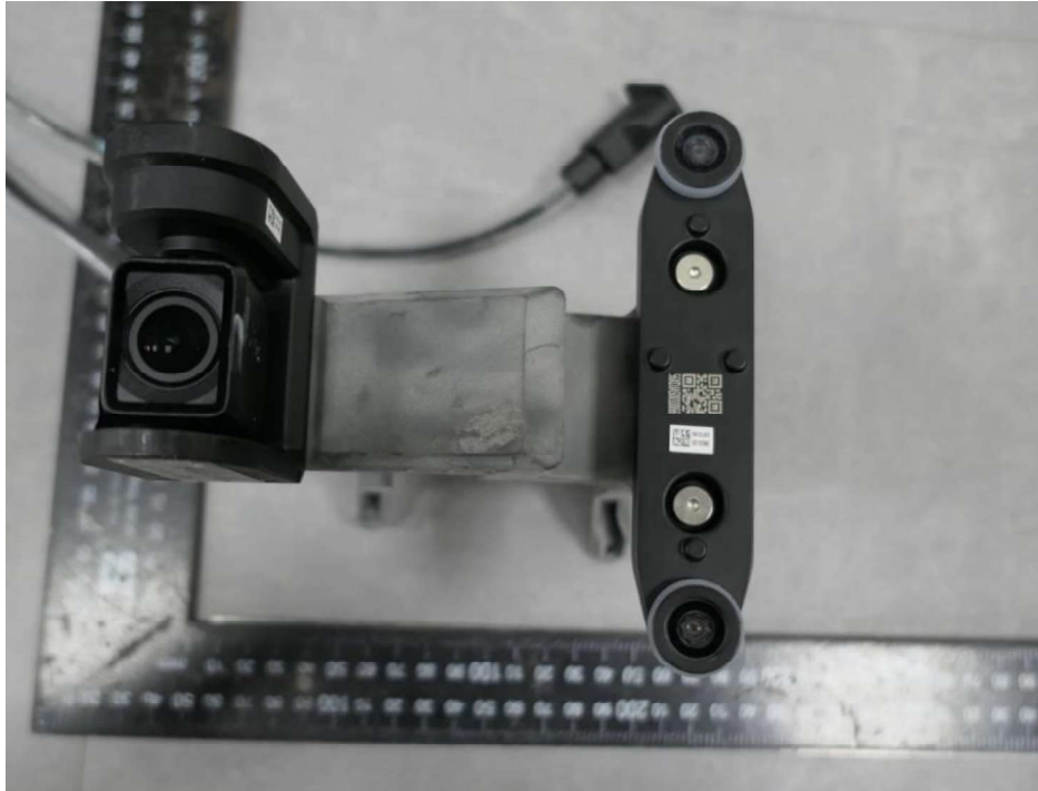
Fig. 27: Front vision system and FPV camera view -2 (for both models)
