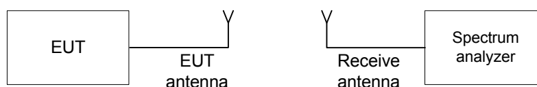
Figure 7.1.1 The 20 dB bandwidth test setup
