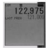
From the example above, the PJ2+ COM is receiving 122.975 MHz with the last frequency being 121.000 MHz. To manually enter a desired frequency such as 118.700 MHz, enter 1 1 8 7 0 0 using the numeric keypad. As each digit is entered, the flashing cursor moves to the next digit. Six digits may be required to select a frequency.
