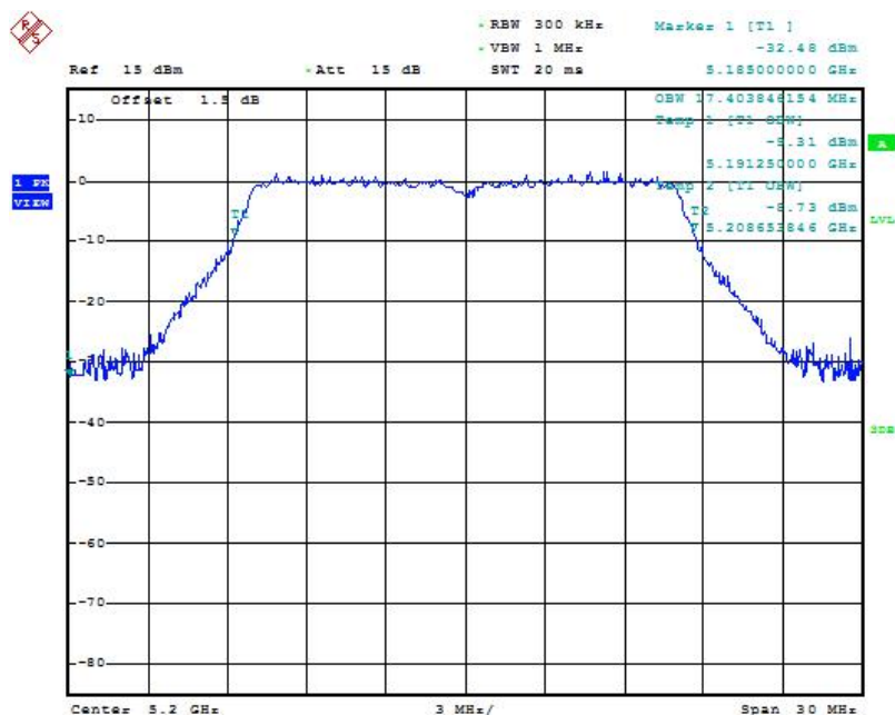
Fig. 9 99% Occupied Bandwidth (802.11a, 5180MHz)
