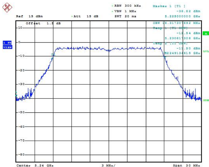
Fig. 13 99% Occupied Bandwidth (802.11n-HT20, 5200MHz)
