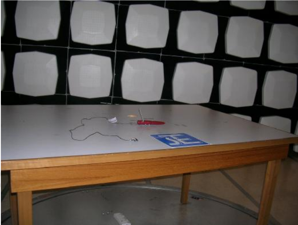
Measurement of Radiated Emission Test Set Up
