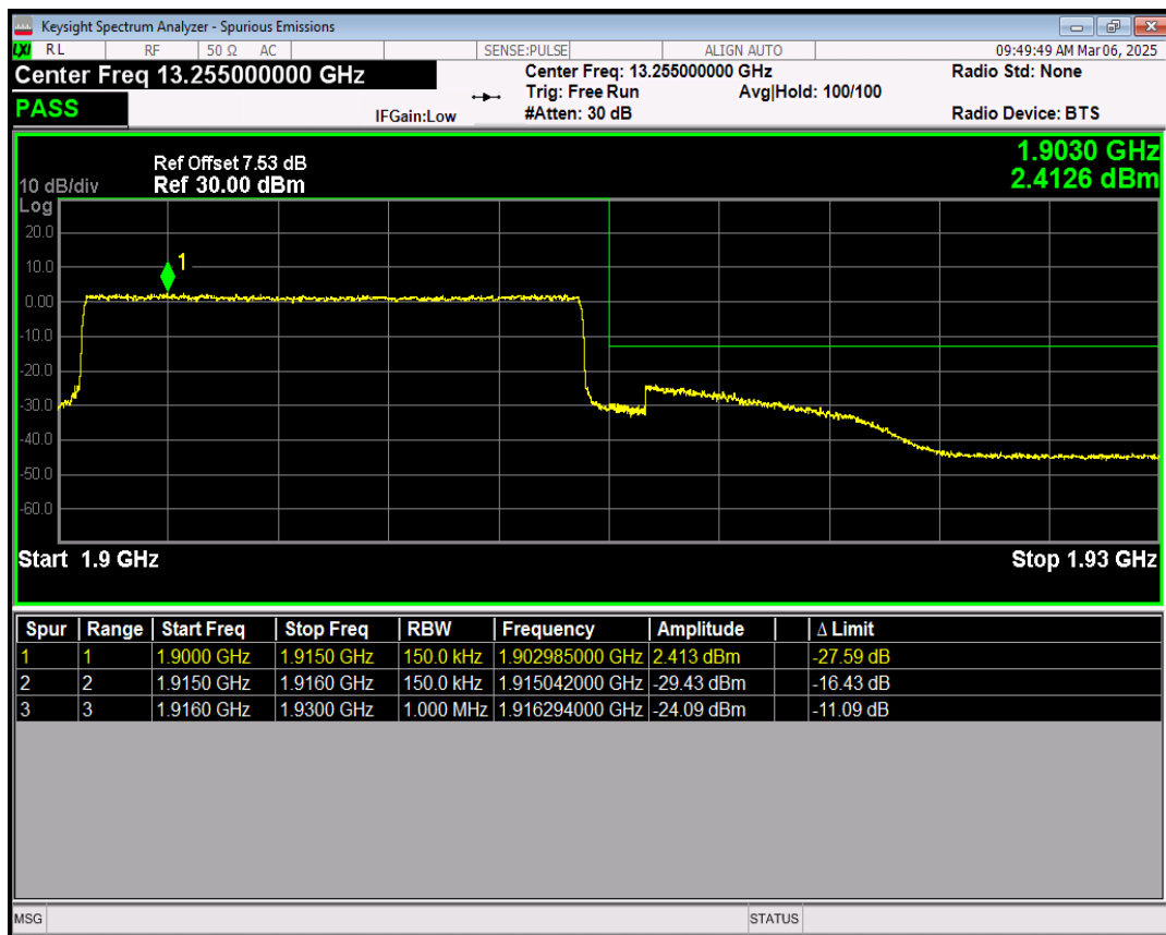
Band25 16QAM BW=15MHz Channel=26615 RB Size=1 Position=#0
