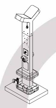
Align the screw holes of the pedestal with the ones in the concrete pier
