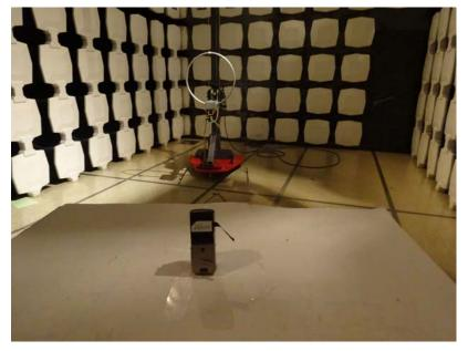
Measurement of Radiated Emission Test Set Up
