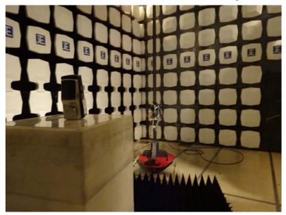
Measurement of Radiated Emission Test Set Up
