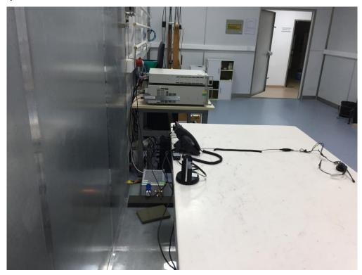
Test Mode 1: Power by adapter #1 and Communication with another IP Phone Description: Radiated disturbance Test Setup for 30MHz ~ 1GHz
