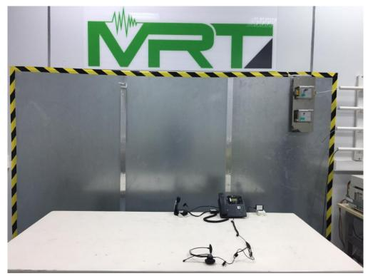
Test Mode 1: Power by adapter #1 and Communication with another IP Phone Description: Back View of Conducted Emission
