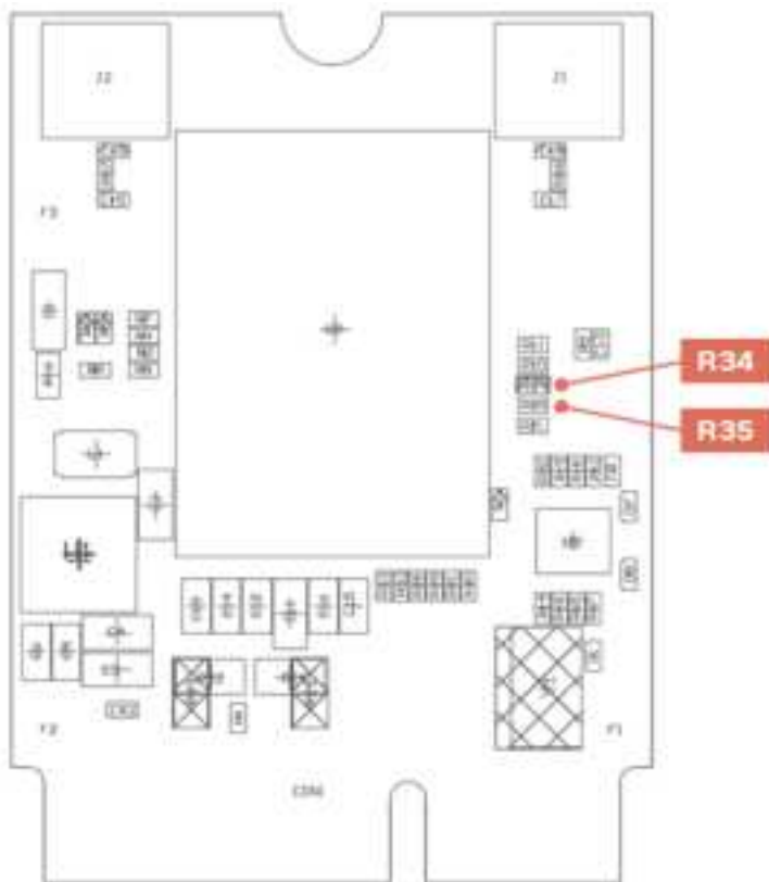
Figure 4: Position of resistors R34 and R35 on M2-MAYA-W1
