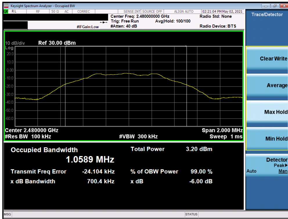
Plot 7-3. 6dB Bandwidth Plot (Bluetooth (LE), 1Mbps, Ch. 39)
