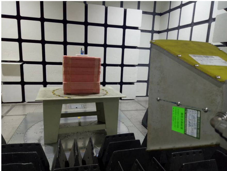
Radiated Emissions View (Above 1 GHz)
