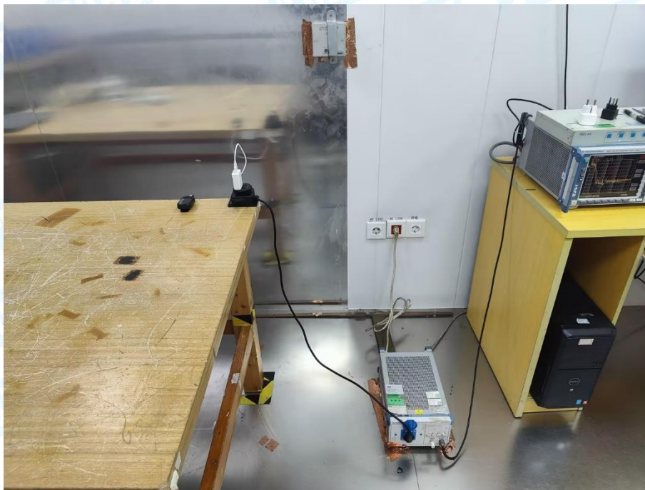
Photo of Setup for Conducted Emission
