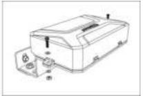
After the hub is secured, remove the hub cover by pressing the tab shown below in **GREEN** and rotating it towards the rear.
