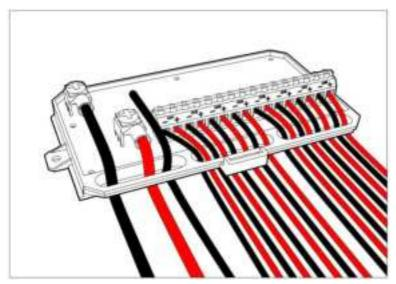
3. Wire Output Channels: Ensure that the main positive power wire is disconnected from the battery before wiring. Wire all desired accessories to the XKcommand hub. Refer to diagram above to see output channel configuration. Channel 1 starts on the left side all the way to channel 8 on the far-right side of the hub. Using a small Phillips head screwdriver, secure wiring for each channel in place. Wiring should pass through the bottom slots as shown in the diagram above.
