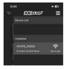
Open the App. It will show "Device Not Connected" on the main screen in red. Go to the Device List by tapping the three lines in the upper right-hand corner. Under the Unpaired list, the new XKcommand controller will be shown. Note-Bluetooth settings may have to be enabled for XKcommand in your phone settings.
