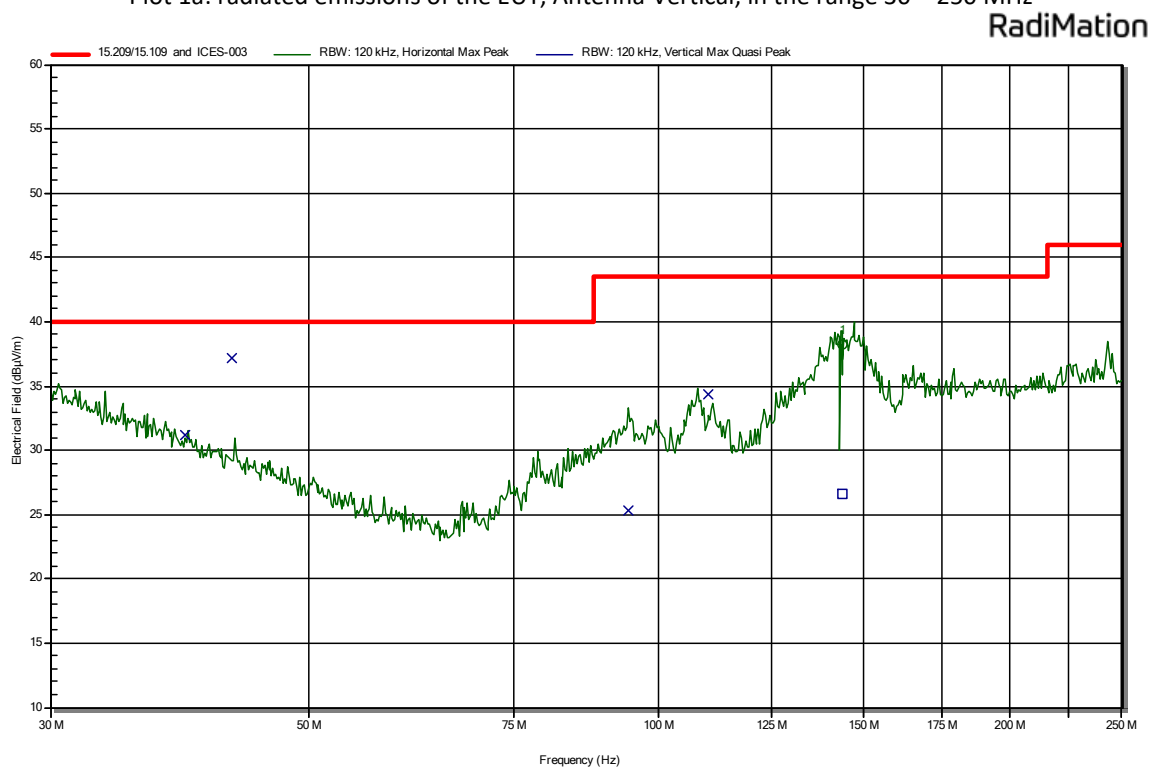
Plot 1a: radiated emissions of the EUT, Antenna Vertical, in the range 30 – 250 MHz
