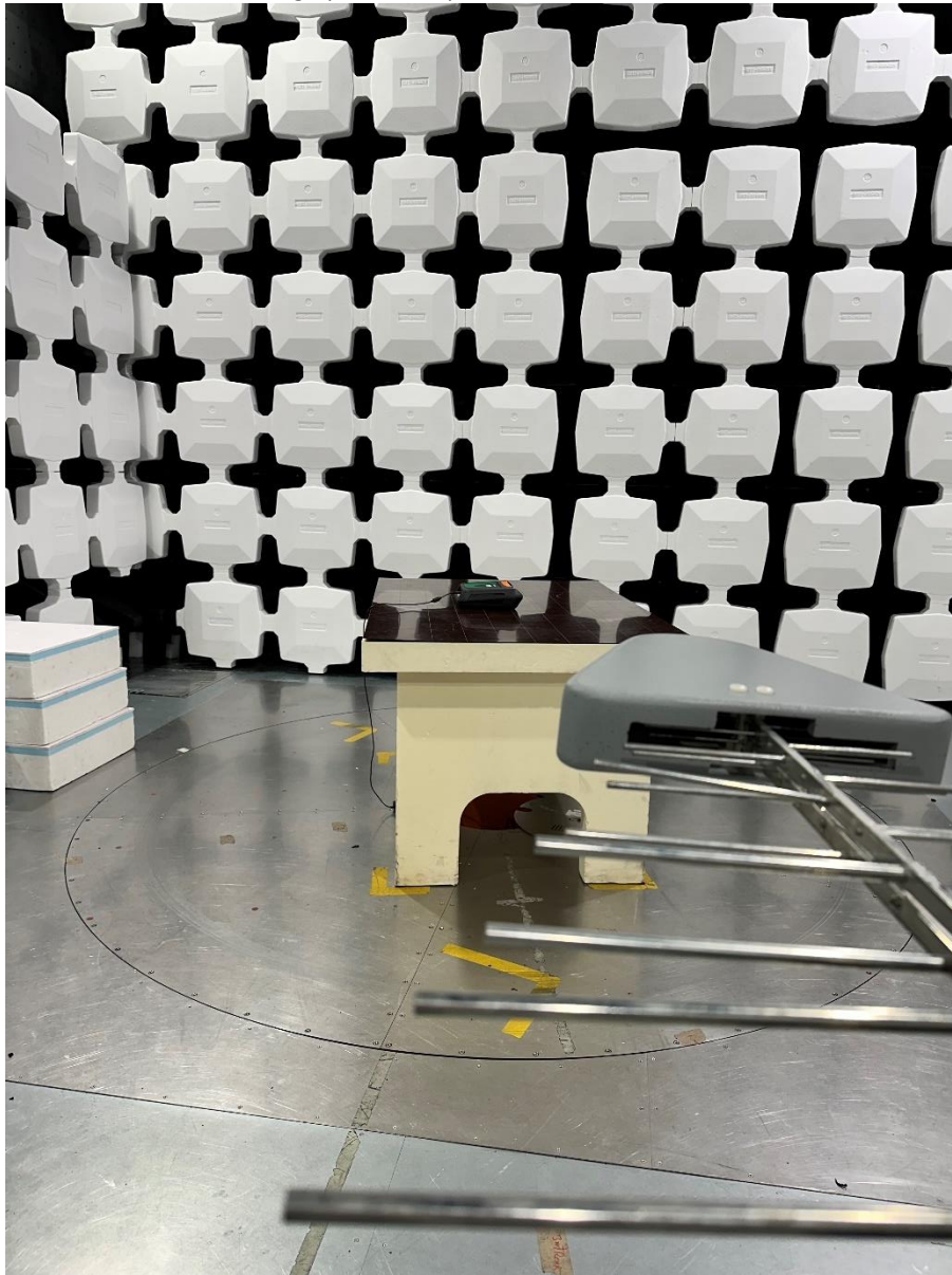
Photo 2 Photograph test setup radiated emissions 250-1000 MHz
