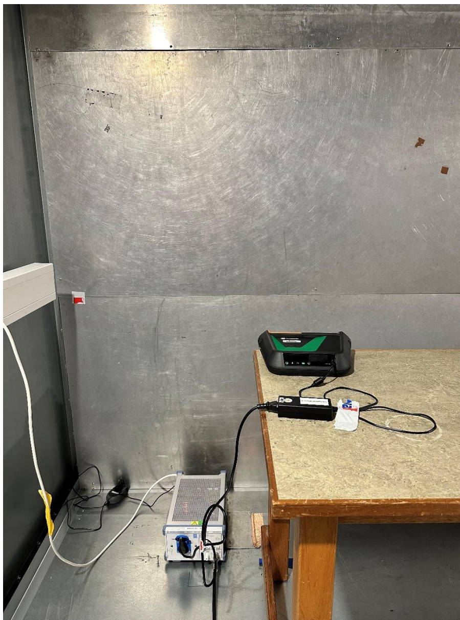
Photo 4: Photographs AC Power Line conducted emission
