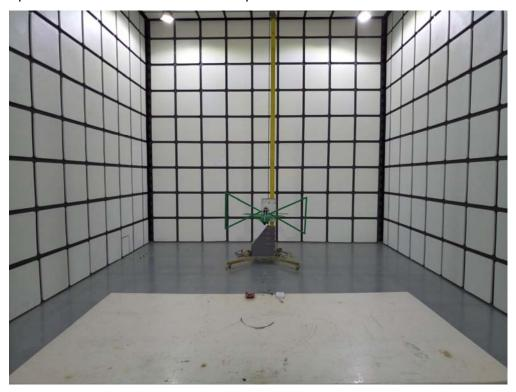
Description: Radiated Emission Test Setup for 1~18GHz
