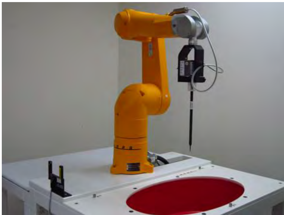
Fig.1 Photograph of the SAR measurement system
