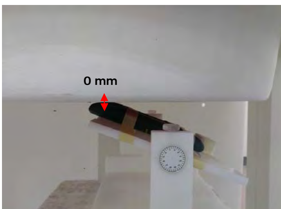
Fig.4 EUT Back side_curve to flat phantom
