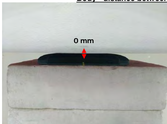
Fig.3 EUT Back side to flat phantom
