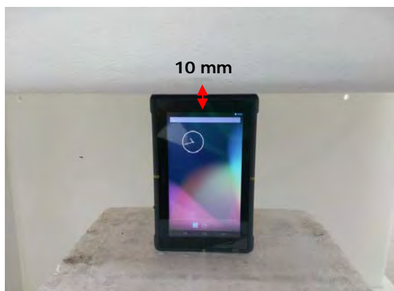
Fig.7 EUT Left side to flat phantom
