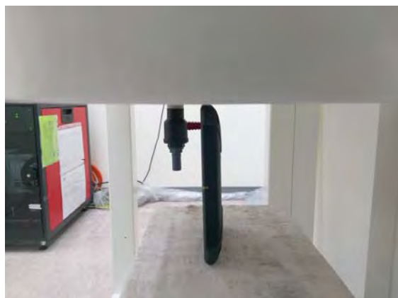
Fig.7 EUT Left side to flat phantom
