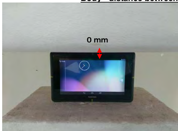
Fig.6 EUT Top side to flat phantom
