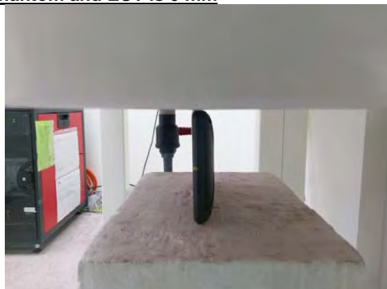
Fig.6 EUT Top side to flat phantom
