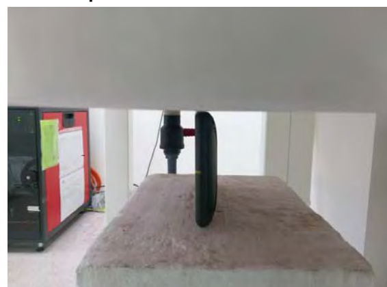
Fig.5 EUT Bottom side to flat phantom
