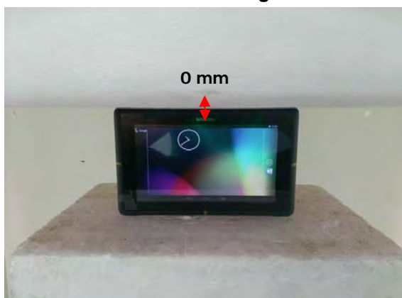
Fig.5 EUT Bottom side to flat phantom
