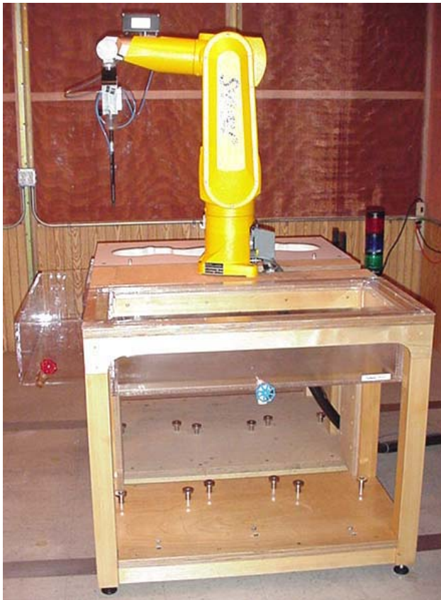
DASY4 SAR Measurement System with validation phantom
