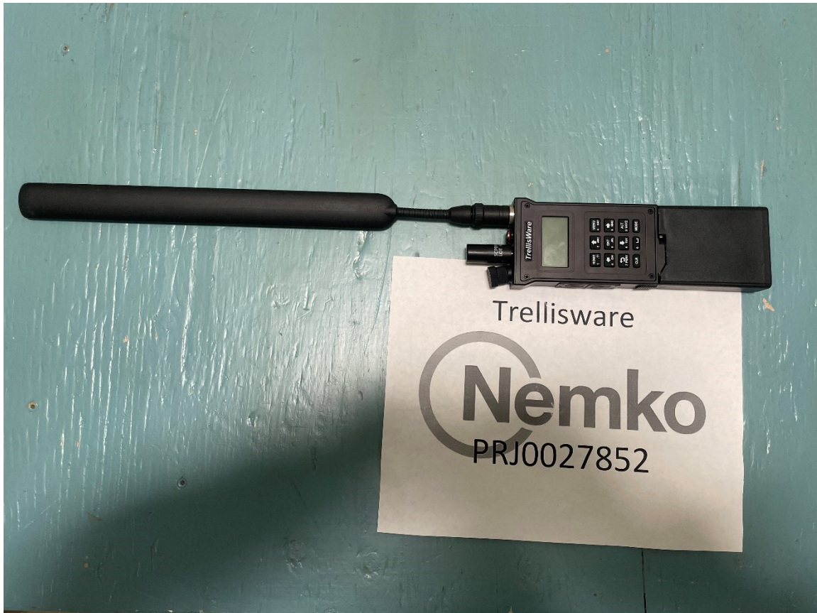
Figure 1 – Test setup showing antenna, antenna connector and battery supply.
