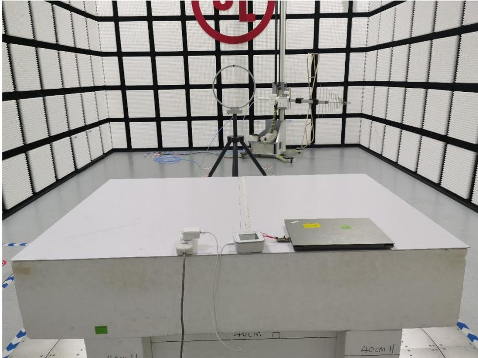
Radiated Disturbance Setup (Above 1 GHz – X axis)
