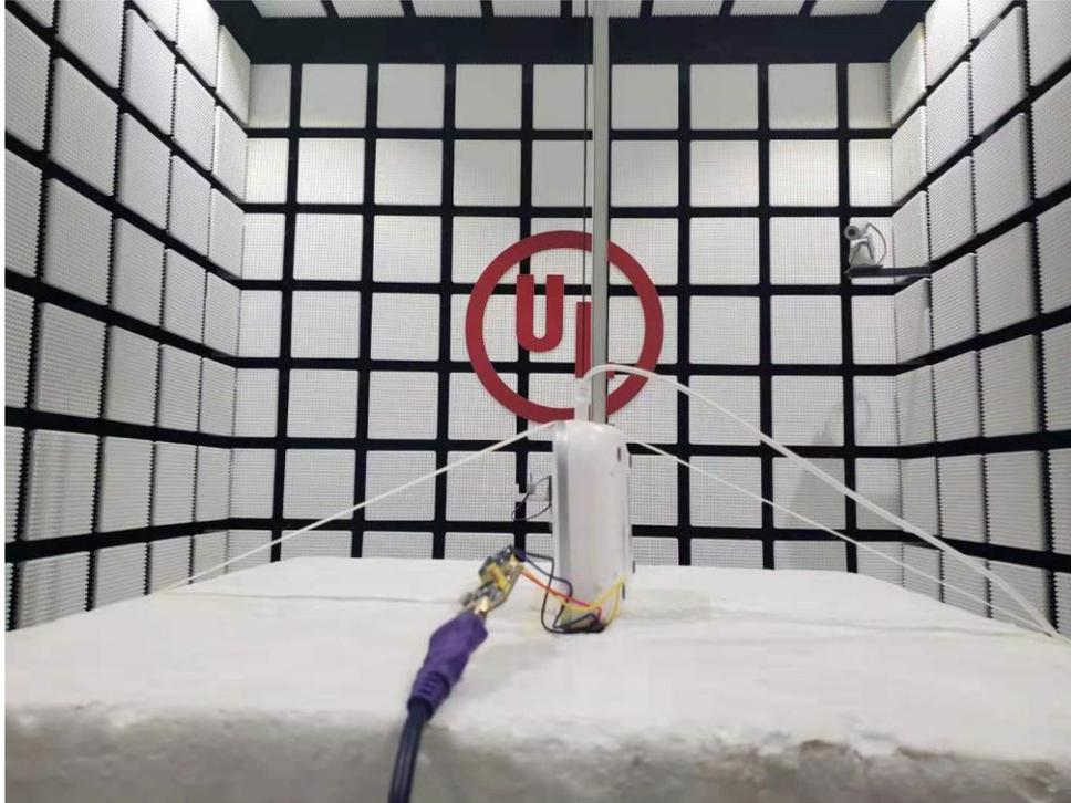
Radiated Disturbance Setup (Above 1 GHz – Z axis)
