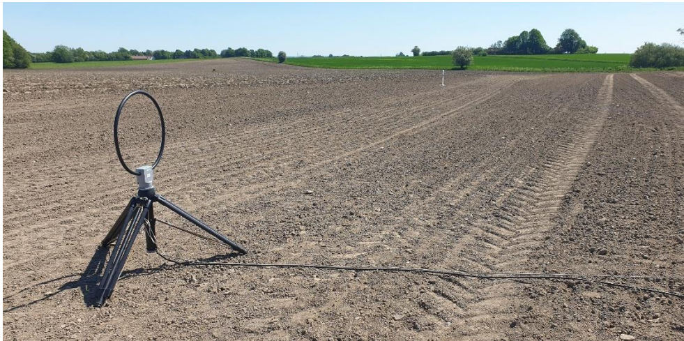
Photo 10. Radiated emission test setup at OATS. 9 kHz – 30 MHz
