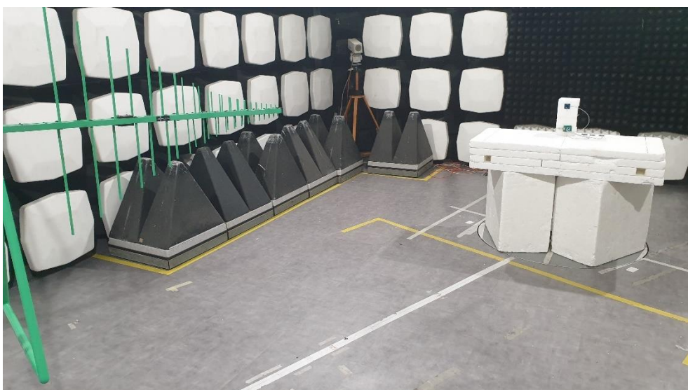
Photo 12. Radiated emission test setup in SAC. 30 - 1000 MHz.
