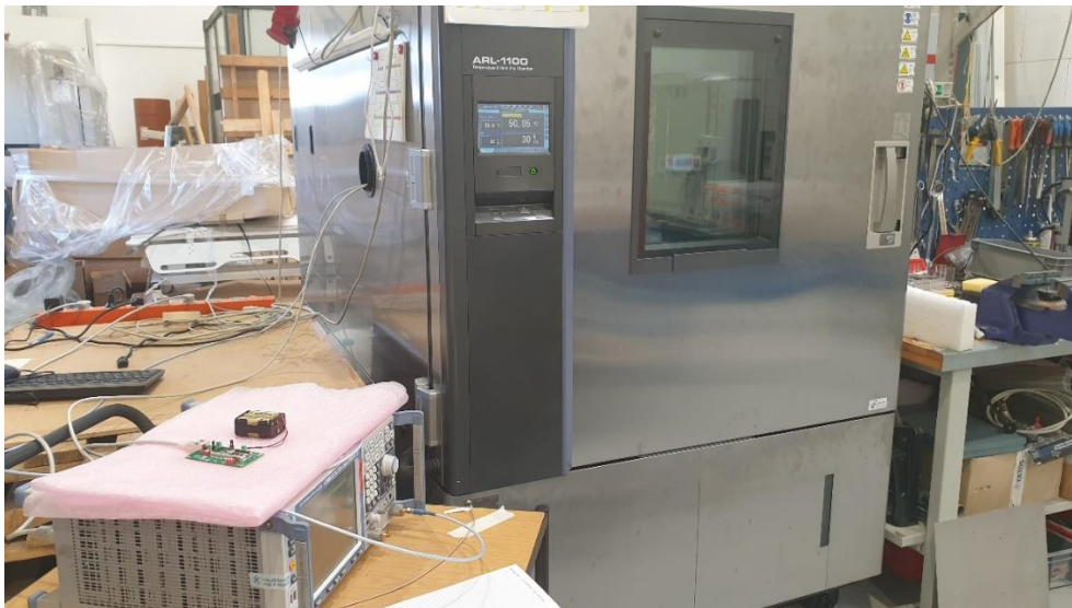
Photo 7. Frequency stability under temperature variation test set up.
