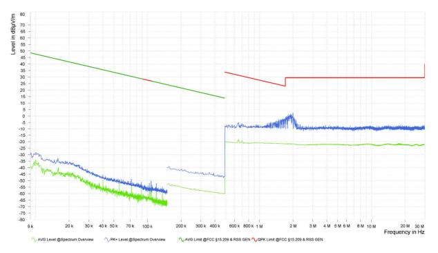
Spurious emissions from 9 kHz to 30 MHz (operation mode 4, position 1):
