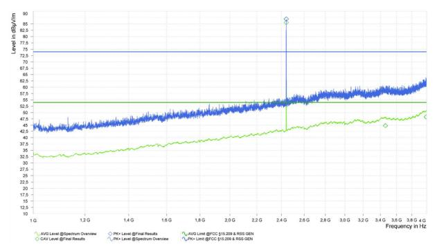
Spurious emissions from 1 GHz to 4 GHz (operation mode 2):
