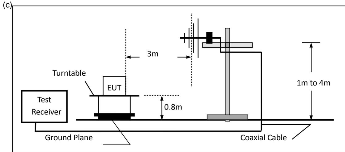
(c) For radiated emissions above 1000MHz
