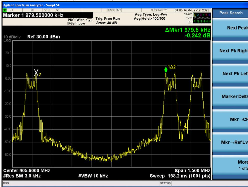
(1Mbps) Channel Separation plot on channel 52-53
