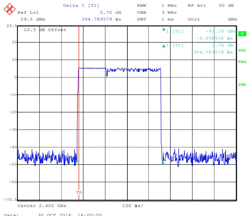
**Pulse time, Middle Channel, 2DH1**
