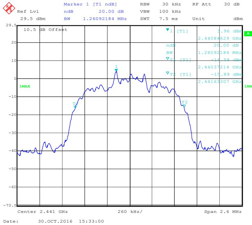
**EDR ( $\pi/4$ -DQPSK): High Channel**
