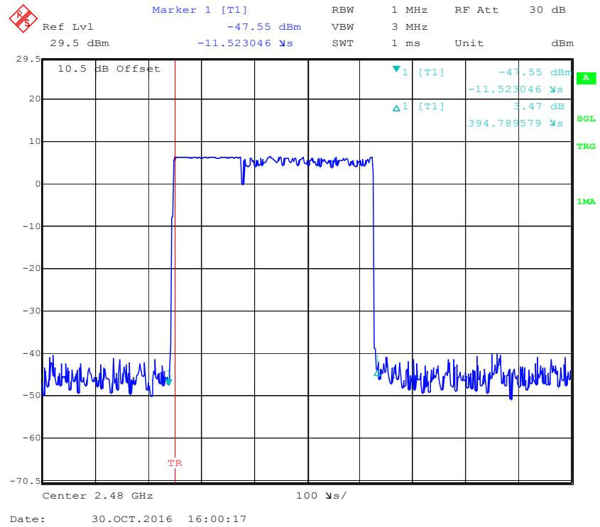
**Pulse time, Low Channel, 2DH3**
