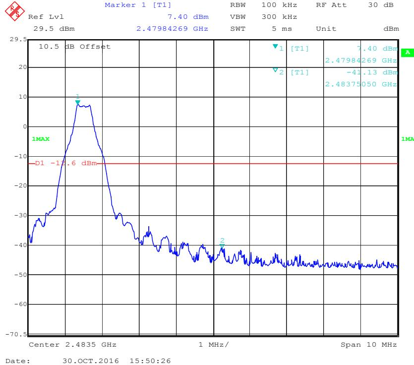
**EDR ( $\pi/4$ -DQPSK): Band Edge-Left Side**
