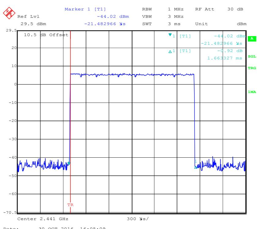
**Pulse time, High Channel, 2DH3**
