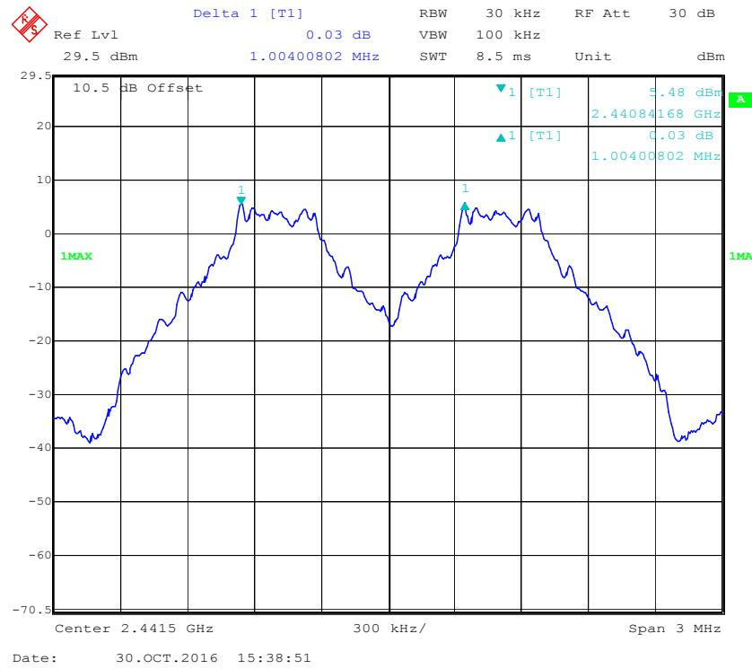
**BDR (GFSK): High Channel**
