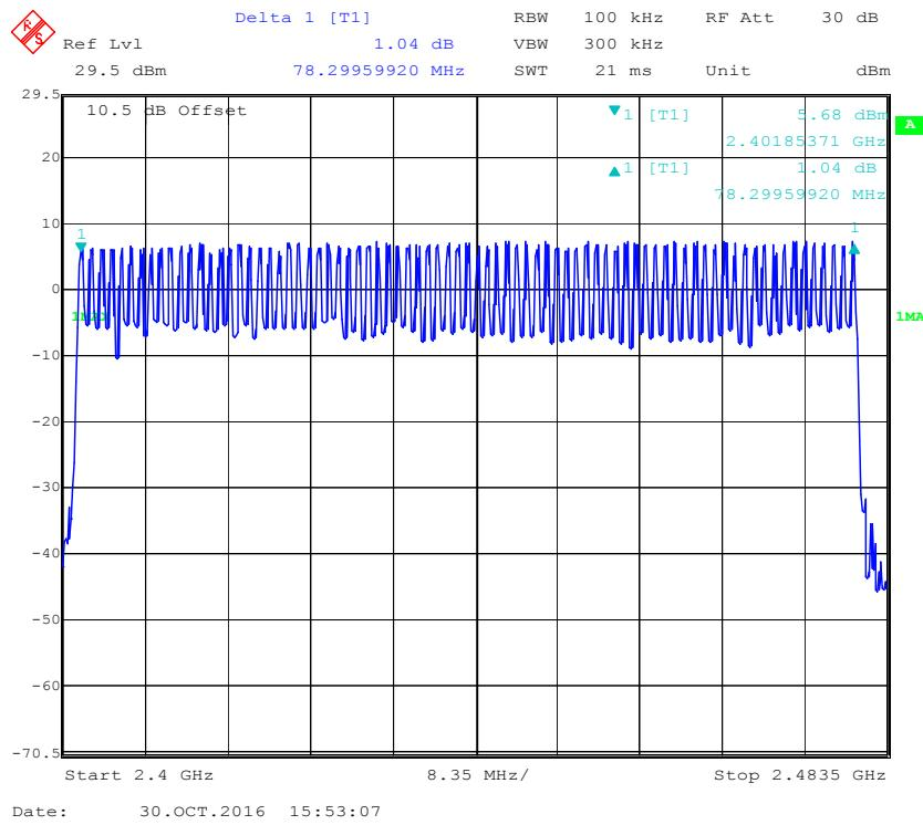
**EDR ( $\pi/4$ -DQPSK): Number of Hopping Channels**
