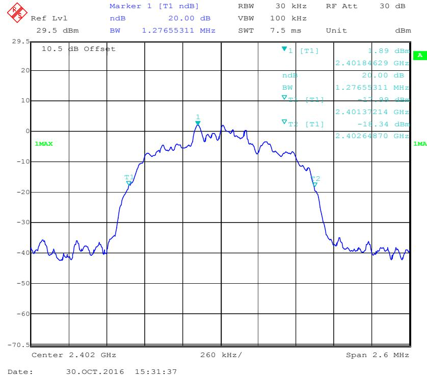
**EDR (8DPSK): Middle Channel**
