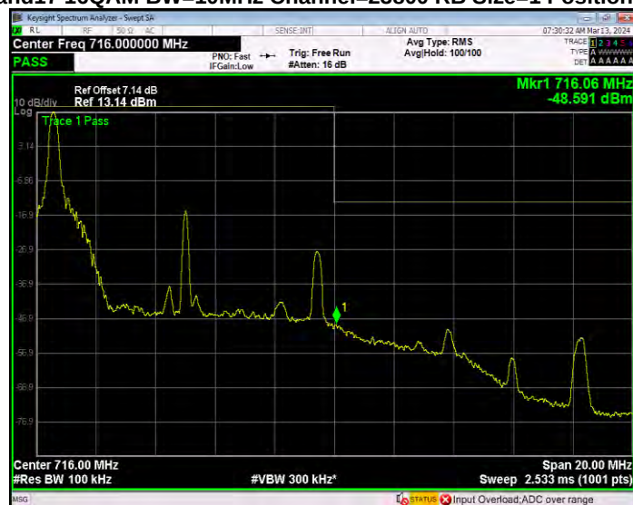
Band17 16QAM BW=10MHz Channel=23800 RB Size=1 Position=#0
