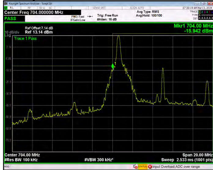
Band17 16QAM BW=10MHz Channel=23780 RB Size=50 Position=#0
