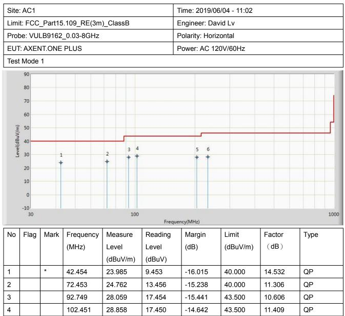
Note: Measure Level ( $dB\mu V/m$ ) = Reading Level ( $dB\mu V$ ) + Factor (dB)
