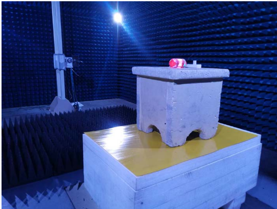
Photo of Radiated Emission Measurement Above 1GHz
