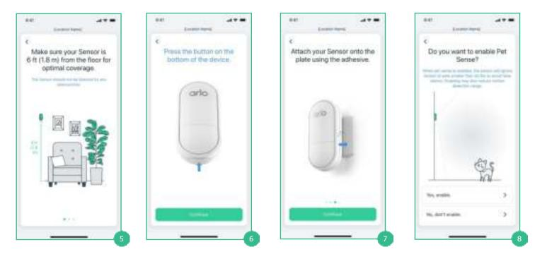
Step 6 Press the sync button on the bottom of the Sensor, then select 'Continue' to proceed.
