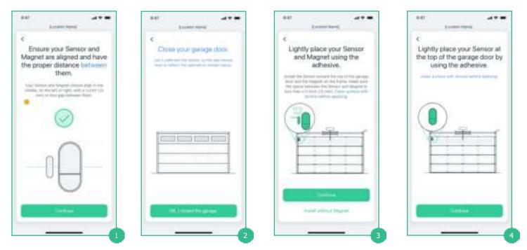
Step 1 Ensure both the Sensor and Magnet are vertical and aligned  $\frac{1}{2}$  inch or 12 mm between one another.
