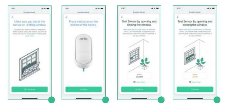
Step 7 & 8 Open and Close the window to verify if the status is accurate. Select 'Continue if it is correct or 'Need help?' if it is incorrect.
