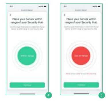
Step 4 & 5 The circle will appear green if the Sensor is within an acceptable range of the Security Hub. If the circle is red, move the Sensor closer to the Security Hub.
