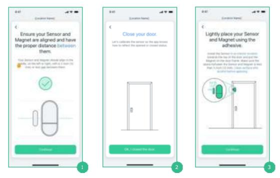
Step 1 Ensure both the Sensor and Magnet are vertical and aligned ½ inch or 12 mm between one another.
