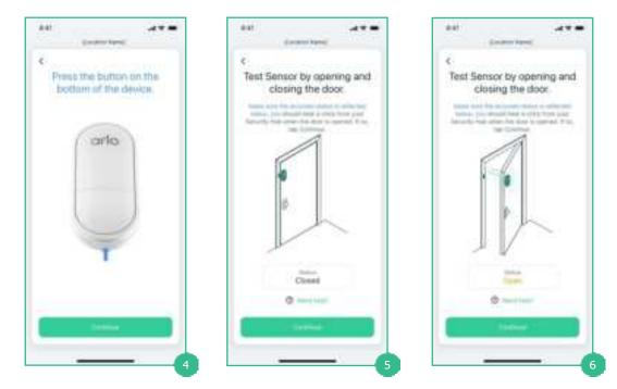
Step 5 & 6 Open and Close the door to verify if the status is accurate. Select 'Continue if it is correct or 'Need help?' if it is incorrect.
