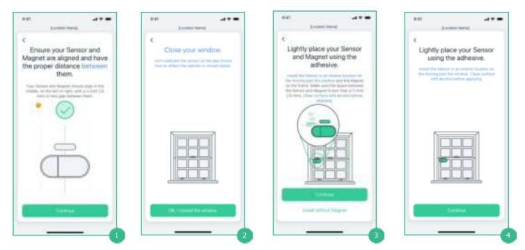
Step 1 Ensure both the Sensor and Magnet are vertical and aligned 1/2 inch or 12 mm between one another.
