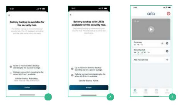
Step 1 Once the Backup Battery has been connected to the Security Hub, wait for the LTE backup to activate.
