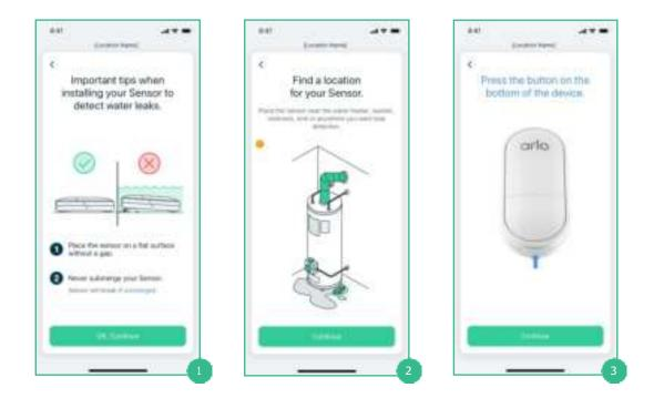
Step 2 Determine a location for the Sensor to detect water leaks.
