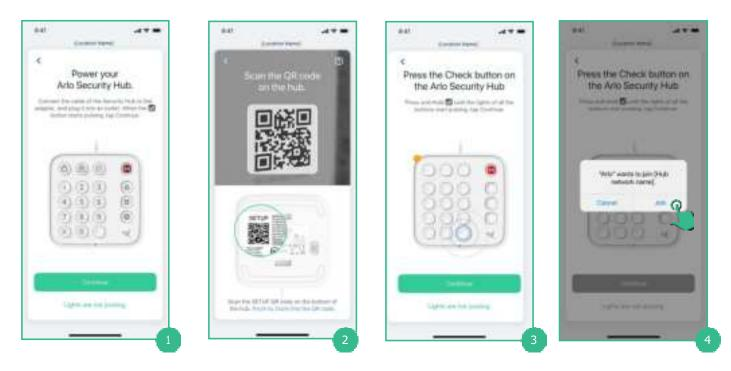
Step 1 On the bottom of the Security Hub, locate and scan the QR code. Step 2 Wait until only the 'check' button LED flashes before selecting 'Continue'.
