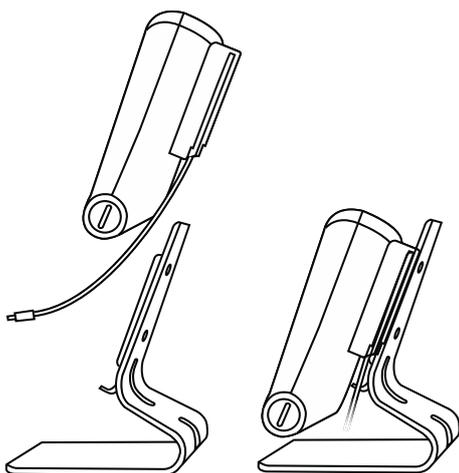
4. Insert the USB cable into the Cable Clips.
