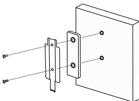
2. Insert the screws in the holes in the Holder Rail and Wall Mount Pad and screw it to a solid surface.
