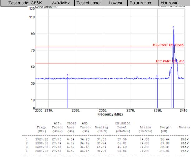
Remarks: 1. Emission Level= Antenna Factor + Cable Loss - Amp Factor + Reading.
