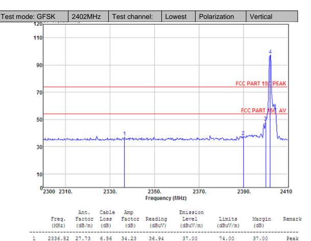
emarks: 1. Emission Level= Antenna Factor + Cable Loss - Amp Factor + Reading.
