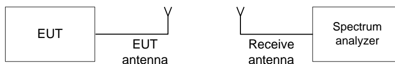
Figure 7.2.1 Carrier frequency separation test setup
