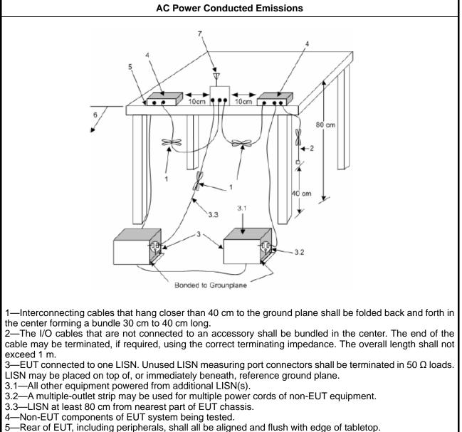
6—Edge of tabletop shall be 40 cm removed from a vertical conducting plane that is bonded to the ground plane.
