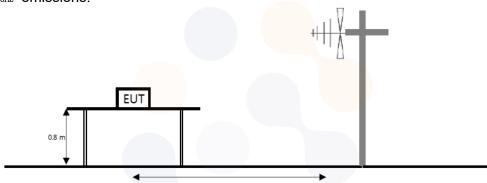
The diagram below shows the test setup that is utilized to make the measurements for emission from 1 to the tenth harmonic of the highest fundamental frequency or to 40 to emissions, whichever is lower.
